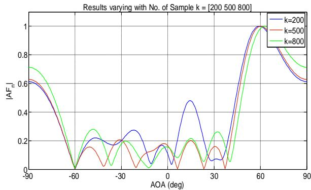
**Fig.6.** Linear Array beamforming Pattern at  $N = 8$ , at  $k = 200,500 \& 800$
