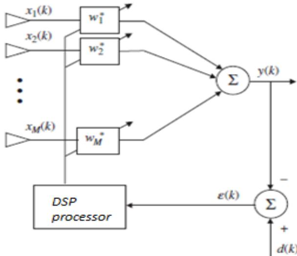
Fig. 1. Showing adaptive processing of Antenna array system [3].
