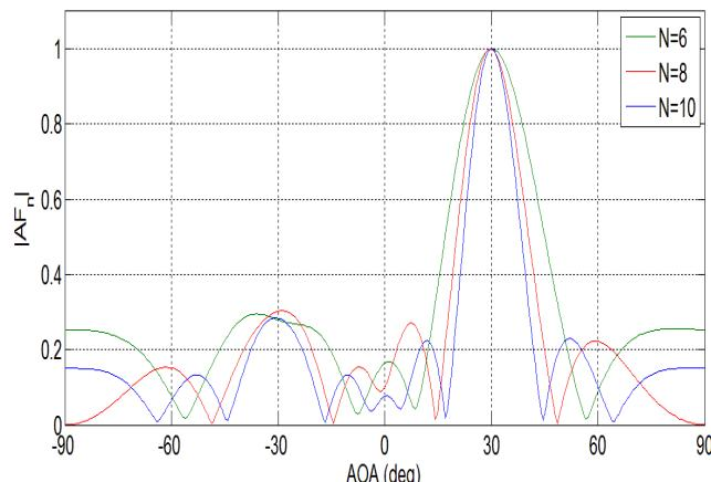
**Fig 8..** Linear Array beamforming Pattern at  $d = 0.5$  &  $N = 6, 8$  and=  $10$
